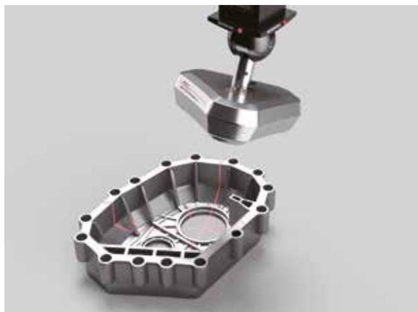
Non-contact laser probes require dramatically less measurement time compared to contact (scanning) probes. Scanning from three directions at once enables simultaneous measurement of the top and side faces, which means less repositioning is required for efficient measurement of even the most intricate workpieces.
