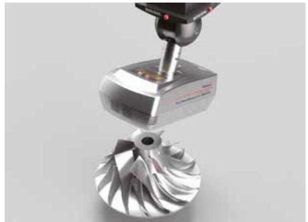
Impellers can be measured using a highly robust non-contact laser probe that reduces multiple reflections. Just as accurate as contact probes, this laser scanner offers high geometric reproducibility.
