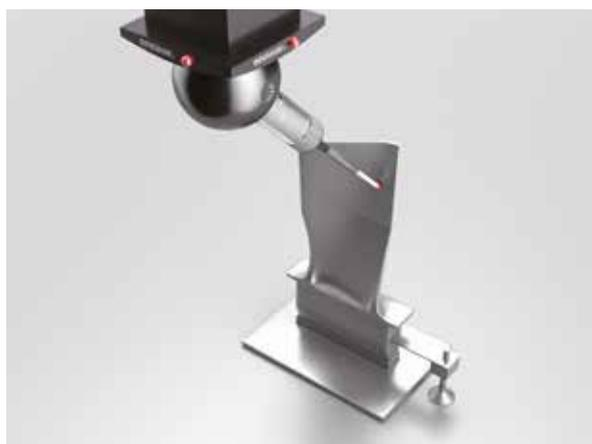
The cross-section of an aircraft engine turbine blade can be measured using a compact, high-accuracy scanning probe that can measure workpieces usually susceptible to large errors, such as castings, quickly and reliably.
